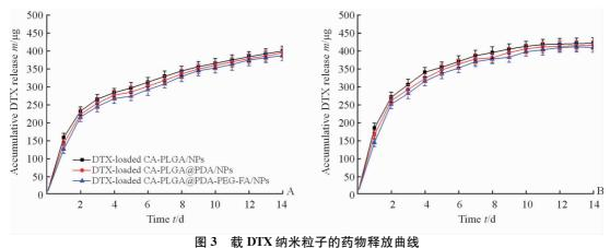
Fig 3 In vitro drug release profiles of DTX-loaded nanoparticles
