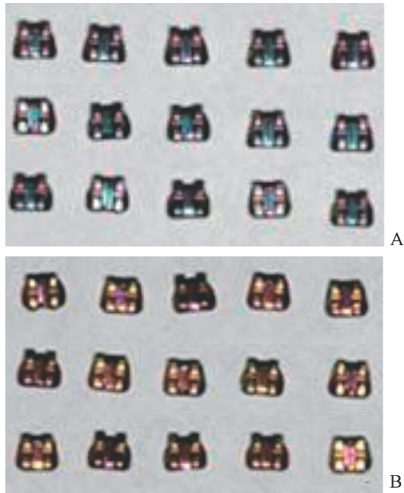
图 2 退火前(A)、后(B) \text{TiO}_2\text{-}_x\text{N}_x 薄膜托槽 Fig 2 Nitrogen-doped \text{TiO}_2\text{-}_x\text{N}_x films on brackets before(A) and after(B) annealing
